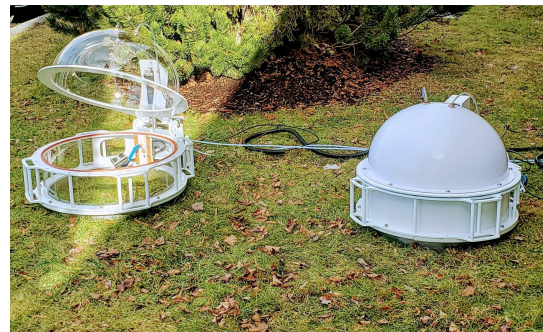
The eosAC-LT (left) and eosAC-LO (right) soil gas flux chambers installed on the front lawn of the Eosense office in Dartmouth, Nova Scotia. The transparent dome of the eosAC-LT allows us to collect measurements of net ecosystem exchange (NEE) alongside measurements of soil respiration using the eosAC-LO with its opaque dome.
